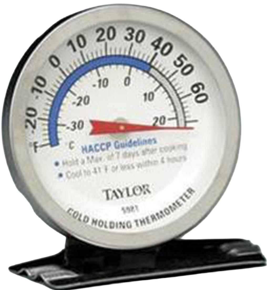
For use in cold holding cabinets where proper holding temperature is critical to food
